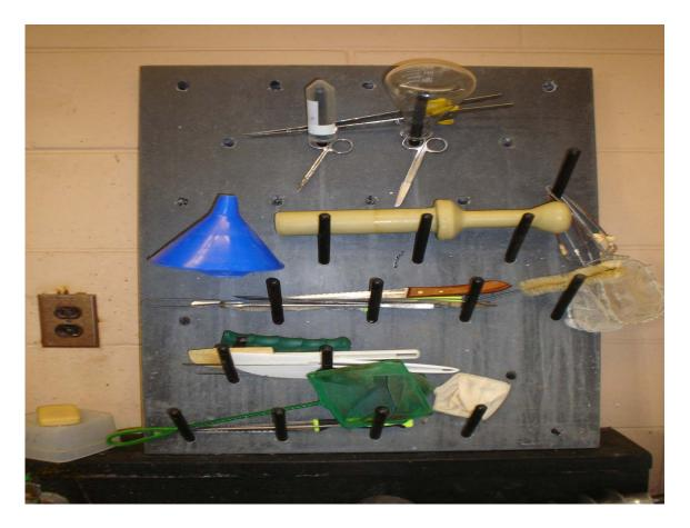
HA #7 – Asbestos-containing transite drying rack
